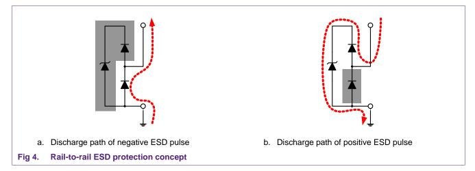
With the rail-to-rail concept, a negative ESD strike on the I/O pin will cause one rail-to-rail diode (the lower diode at the flash sign in <u>Figure 4</u>, left side) to become forward biased, thereby transferring the ESD strike through the lower diode to ground.
