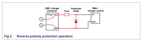
The positive voltage supplied to the GND input of the charger can pass through the forward biased protection diode and the protective fuse, back to the charger negative pole. In this concept the protection diode needs to be able to conduct high currents only until the fuse clears. Fast reacting fuses can clear in 100 ms. Section 3.4 describes protection diodes that are able to conduct up to 5 A for the necessary period of time.
