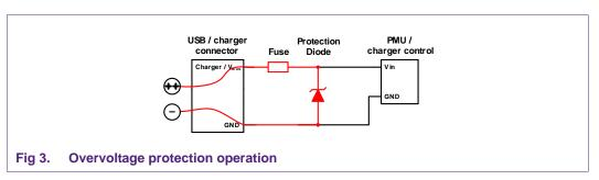
If not already present for reverse polarity protection (see <u>Section 3.1</u>), a fuse or Positive Temperature Coefficient (PTC) element should be placed in the supply path. This limits the current if, for example, defective charger supplying the primary voltage is connected and the continuous current that passes via the Zener diode exceeds the limit imposed by the maximum power dissipation.
