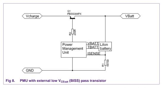
In switched current sources the low  $V_{CEsat}$  transistor is used in saturation mode, the minimum gain should be taken into account, at 1 A the gain of the PBSS304PX is 200. Therefore a minimum base current of 5 mA is needed, to ensure we will set the base current to 10 mA. The additional resistor R2 should limit the maximum current of the drive stage.
