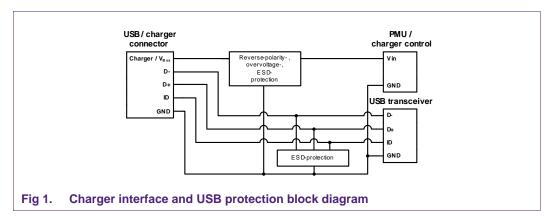
As shown in Figure 1 a complete protection solution for the USB and charger port consists of two blocks. The first block protects the USB  $V_{BUS}$  or charger interface against reverse polarity and overvoltage. The second block protects the USB data lines and the downstream components against damage from ESD. The subsequent sections illustrate the protection concepts of these blocks in more detail.
