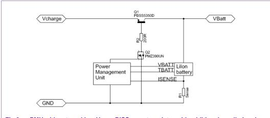
Fig 9. PMU with external low V<sub>CEsat</sub> BISS pass transistor with additional small-signal MOS control transistor
